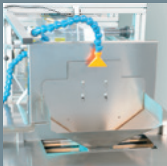
Mobile hopper and antiwrinkle device
